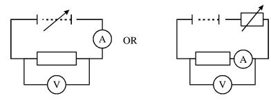
Accept voltmeter across heater and ammeter as well as voltmeter across heater only
